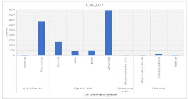
Figure 29 - CUIB Life Cycle Costing (LCC) results in euros per year
